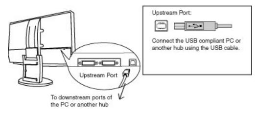
After connecting the USB cable, the USB function can be set up automatically.
